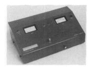
• Lovibond's Automatic Colorimeter measures refined edible oil colors automatically and reads out in Lovibond units, up to 40 yellow and 20 red. The unit measures optical density of samples at two points in the spectrum, approximately equal to the colors of the Tintometer red and yellow filters. The unit is designed to ignore the effect of bubbles and suspended particles. Information: Tintometer Information Service, PO Box 17, Bloomingdale, NJ 07403
