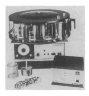
• Shandon Southern Instruments has improved its 2-liter Automatic Tissue Processer to include an optional vacuum embedding unit that plugs directly into the processor. Information: Shandon Southern Instruments Inc. 515 Broad Street, Sewickley, PA 15143.
