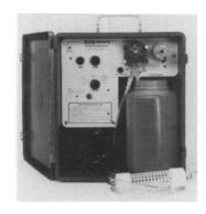
• N-Con's automatic sampler collects samples of sewage or industrial wastes for analysis at a rate from one sample every three hours to eight samples per hour. Volumes collected are infinitely adjustable from 10 ml to 300 ml. Information: J.S. Beach Jr., N-Con Systems Co., Inc., 308 Main St., New Rochelle, NY 10801.
